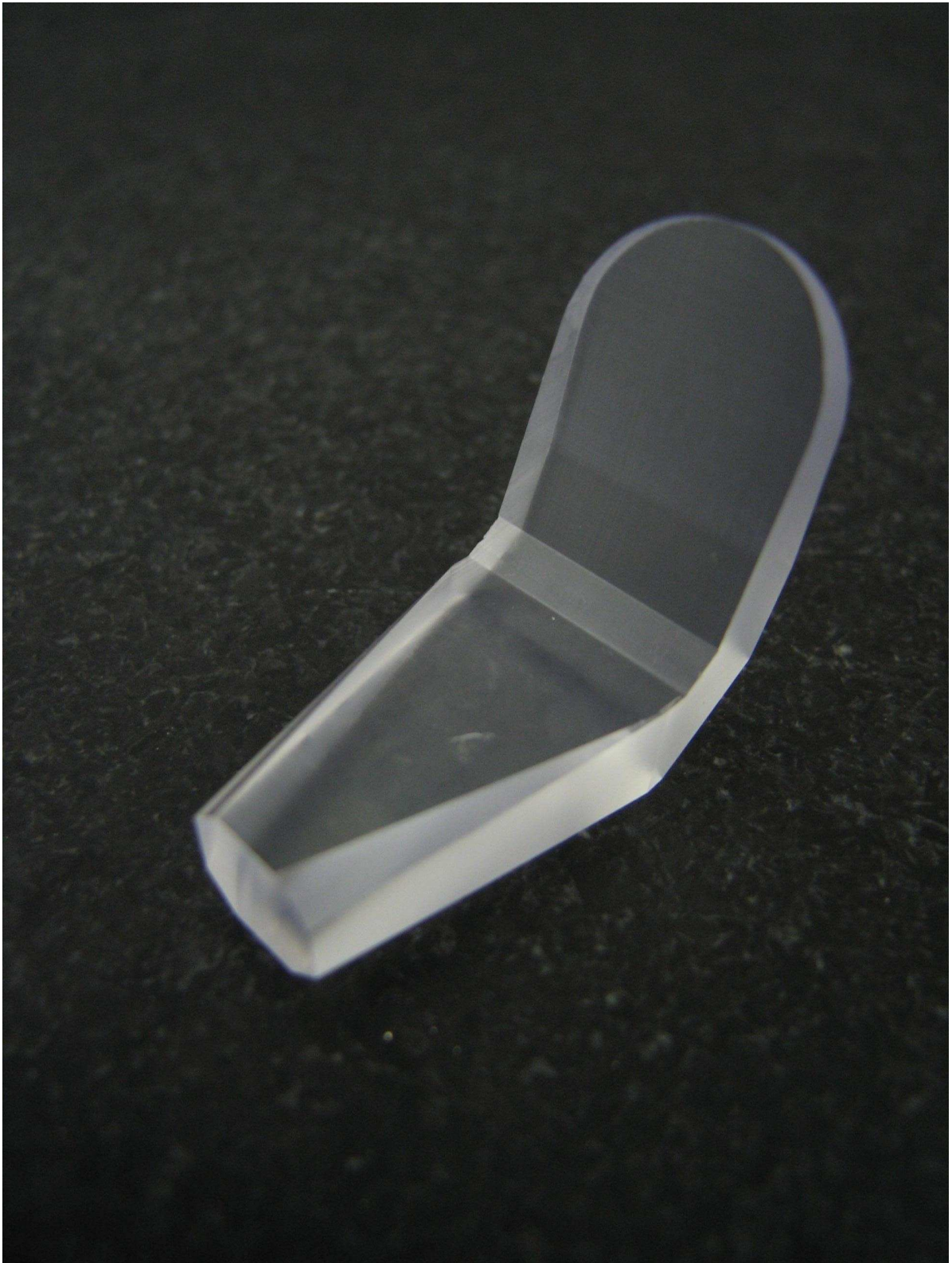
Figure 3.9: A single degrader scintillating finger. The tip region is the scintillator and the rest is made up of a light guide.
