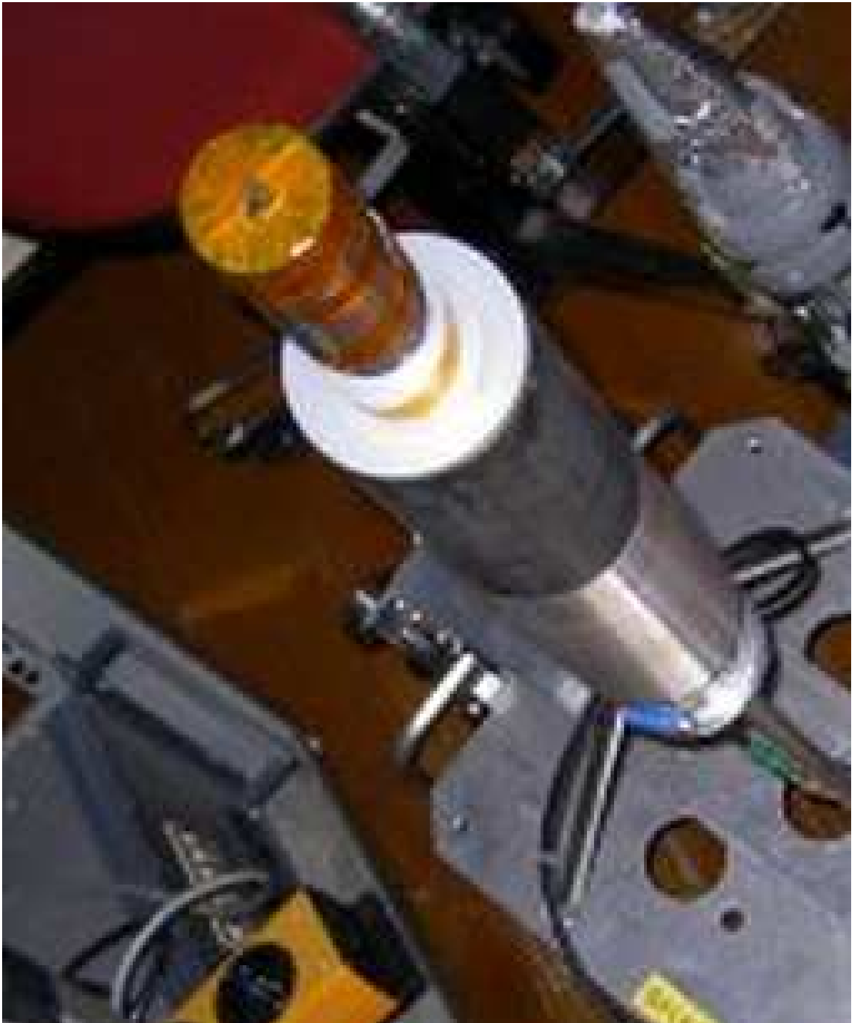
Figure 3.12: Wrapped and mounted active target counter. Behind it is an air light guide and then the photomultiplier tube.
