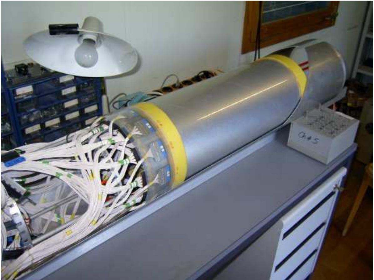
Figure 3.14: The outer multi-wire proportional chamber. The white cables are the cathode signal readout.
