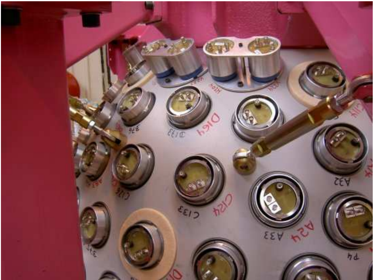
Figure 3.17: Close up of exterior of CsI crystal housing, the circles are PMT bases.
