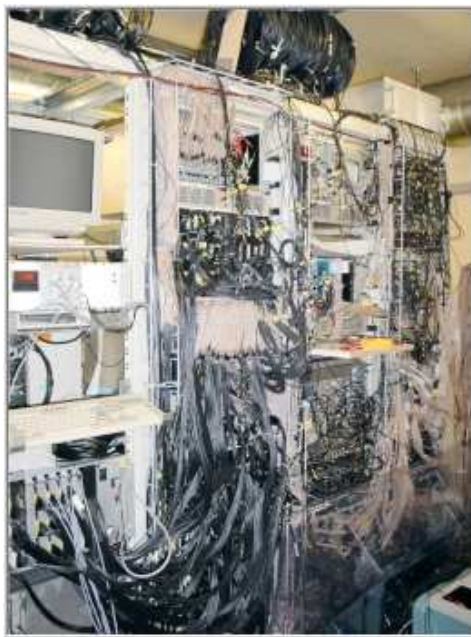
Figure 5.14: A photograph of the PEN electronics hut. The trigger system is located on the rightmost section. Below that behind plastic shielding are the raw CsI signal cables. The middle section of the racks contain the bulk discriminators and the bottom of the leftmost rack contains the FASTBUS modules. The left-hand section contains the slow control systems.
