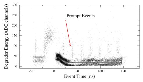
Figure 1: Degrader energy vs. event time for all events in the  $\pi^+ \to e^+ \nu$  DST. Prompt events which are in time with the beam particles deposit more energy in the degrader.
