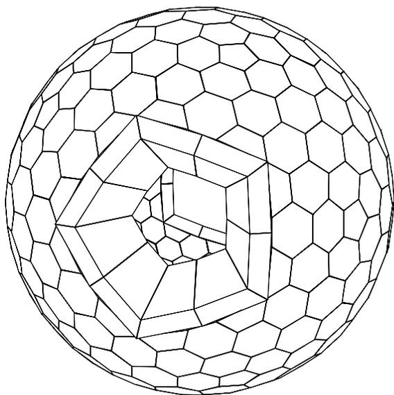
Figure 3: (left) A view showing the geometry of the pure CsI shower calorimeter. The sphere is made up of 240 elements, truncated hexagonal, pentagonal, and trapezoidal pyramids; it covers about 80% of  $4\pi$  in solid angle.
