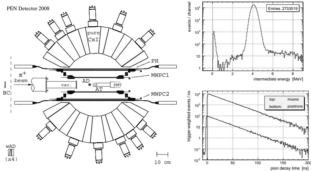
Fig. 1. Left: Cross section drawing of the PEN detector system. Right: Energy distribution of the intermediate muon in the  $\pi \rightarrow \mu \rightarrow e$  decay chain, extracted from AT waveform data (top). Time dependence of the  $\pi \rightarrow \mu$  and  $\pi \rightarrow e$  decays, from the AT waveform data.
