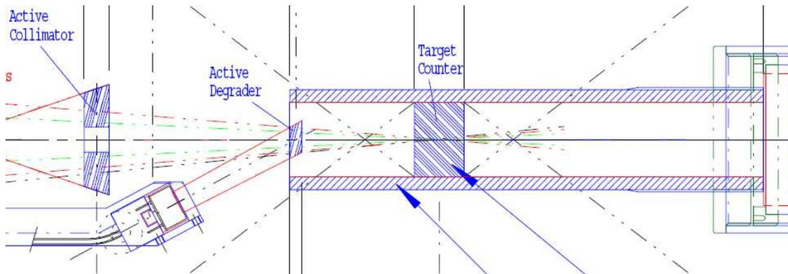
Figure 1: Schematic drawing of the central-region beam detectors redesigned for the 2006 PEN run: the active collimator, degrader, active target (with fast central scintillator and a slow-scintillator cylindrical shield). The upstream Beam tag detector, also redesigned for 2006, is not shown.
