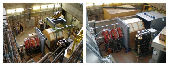
(a) Photograph taken during the assembly of the PEN de- (b) PEN detector system in 2010 with the lead shielding tector system in 2007. house rolled away allowing us to view the thermal house
