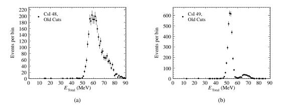
**Figure 4.26:** *Initial CsI energy calibration method for crystals* (a) 48, and (b) 49, *demonstrating the lack of precision in the method for crystal 48.*
