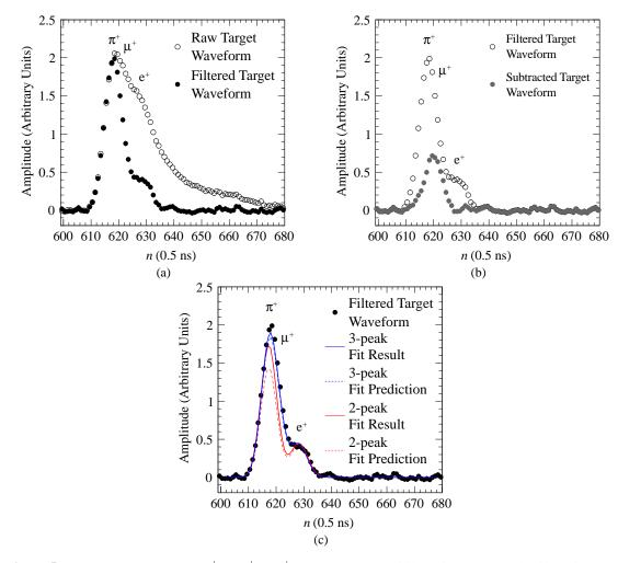
**Figure 5.7:** Target waveform of a  $\pi^+ \rightarrow \mu^+ \rightarrow e^+$  event. (a) raw and filtered waveforms, (b) filtered waveform before and after subtraction of predicted  $\pi$  and e pulses and (c) fits for both the 2-peak and the 3-peak hypothesis.
