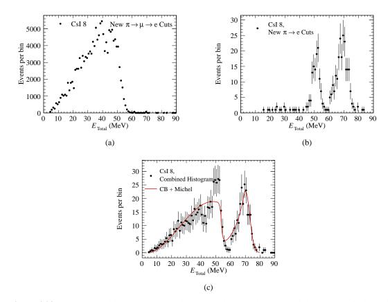
**Figure 4.28:** New CsI Calibration for crystal 8. (a) with cuts selecting Michel events, and (b) with cuts selecting  $\pi \rightarrow e$  events. (c) combination (a) and (b) along with a fit.
