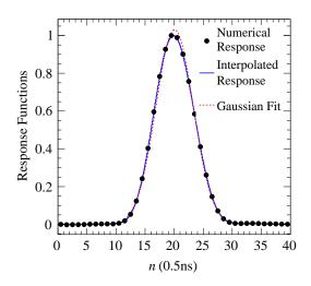
**Figure 5.5:** *Filtered target waveform response function and Gaussian fit, demonstrating a slight discrepancy near the peak.*
