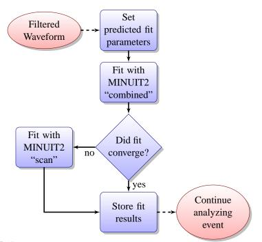
**Figure 5.10:** Waveform fit flowchart demonstrating the check for convergence and the second fit attempt with the "scan" method when the "combined" method fails.
