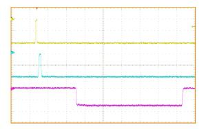
**Figure 3.16:** The  $\pi GATE$  signal for a single event. Top trace = BC, Middle trace = (DR · DL), Bottom trace =  $\pi GATE$ . Vertical scale: 400 mV/div (top), 700 mV/div (middle), 500 mV/div (bottom). Horizontal scale = 50 ns/div.
