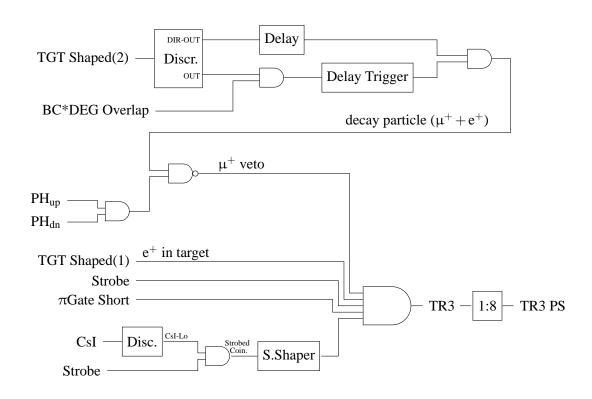
Figure A.11: TR3 (part2) — Muon veto with TR3 triggers.
