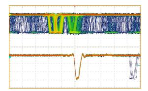
**Figure 3.15:** The BC signal contains three distinct pulses. By aligning the coincidence with the degrader signal one can select the particle (pion, muon, positron – left to right). Top trace = BC, Bottom trace = (DR · DL). Oscilloscope is triggered on (DR · DL). Vertical scale: 300 mV/div. Horizontal scale = 10 ns/div.
