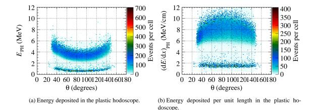
**Figure 6.11:** The plastic scintillator hodoscope is useful for discriminating between positrons with  $dE/dx \sim 1.5$  MeV/cm and protons with  $dE/dx \sim 6.5$  MeV/cm.
